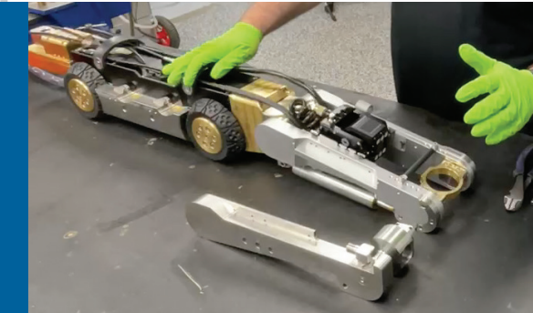
It takes less than 10 minutes to turn your Schwalm Robot into a 2800 bar water jetter.
