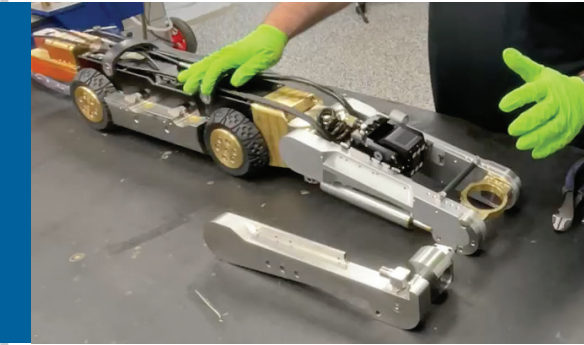
It takes less than 10 minutes to turn your Schwalm Robot into a 2800 bar water blaster.
