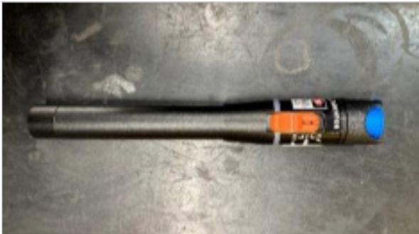
Figure 3: VFL- Visual Fault Locator
